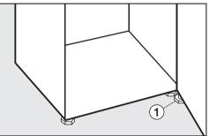
■ **Ensure** that you unscrew adjusting foot ① from the hinge plate until it sits on the floor. Then unscrew the foot by a further 90°.
